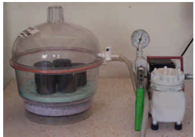
Figure 3-3: Vacuum chamber containing the five containers
