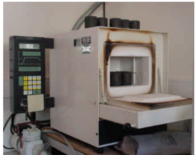
Figure 3-2: The furnace and its electronic controller and the five containers
