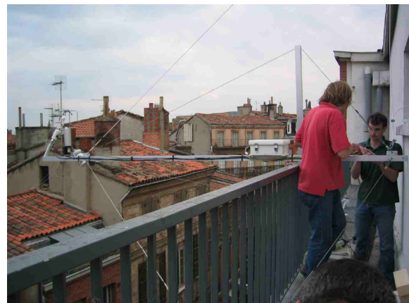
Figure 3 Boom above street to measure canyon top processes
