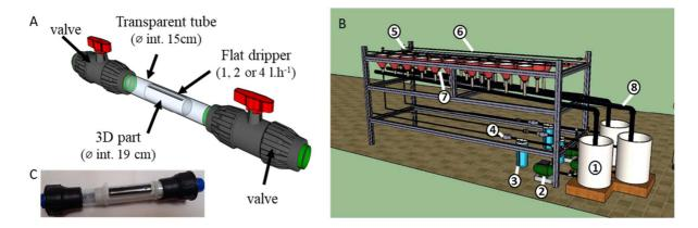
Figure 1. Dripper system (A, C) and test bench (B). The drippers were placed in a transparent tube to enable optical measurements. The test bench was composed of 1. a tank (60l); 2. a water pump; 3. a 0.13mm mesh screen filter; 4. a pressure reducer; 5. a
