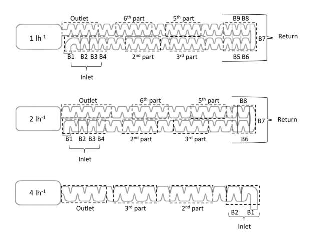
Figure 2. Schematic diagram of the geometric channel from the drippers. The dotted boxes correspond to the study areas. The length and width (in mm) of each baffle are listed in the Table S1 in Supplementary material.
