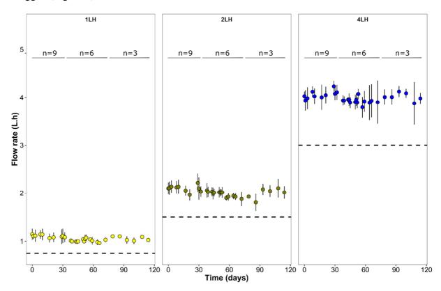
**Figure 3 Mean flow rate (and standard error) according to the dripper type.** The dotted line of discharge of less than 75% corresponds to the limit usually set up to consider that a dripper is clogged. n refers to the number of dripper of the lines.
