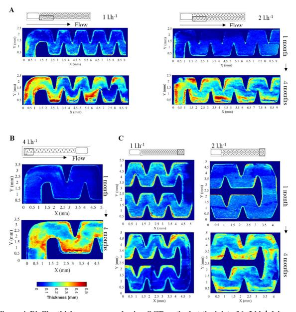
Figure 4. Biofilm thickness measured using OCT method at the inlet of 1, 2 l.h<sup>-1</sup> drippers (A) and 4 l.h<sup>-1</sup> dripper (B) and in the return areas of drippers (C) measured after 1 and 4 months.
