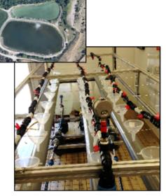
Lab drip irrigation system supplied by reclaimed wastewater
