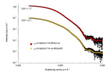
**Figure 3.** Superimposition of SAXS data from <sub>His</sub>-In-*Np*Xyn11A-*Bh*Xyl43-Jo and <sub>His</sub>-In-*Np*Xyn11A-Jo-*Bh*Xyl43 constructs and their structural models calculated with SASREFMX (red and orange line respectively). The data are presented as a plot of Log I(q) in cm<sup>-1</sup> vs. Log q in Å<sup>-1</sup> to magnify the region of small angles.
