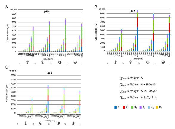
**Figure 5.** Evolution of the concentration of xylooligosaccharides from  $X_1$  to  $X_6$  at (**A**) pH 6, (**B**) pH 7 and (**C**) pH 8 over time determined by HPAEC-PAD. Hydrolysis conditions: 1 nM of enzymes, 37 °C 1% BWX during 24 h. Representation of the average of triplicate experiments (see Figure S6 for details).
