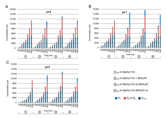
**Figure 6.** Evolution of the concentration of the total reducing equivalent xylose at (**A**) pH 6, (**B**) pH 7, and (**C**) pH 8 over time measured by DNS assay. Integrated with the DNS results, the concentration of xylose and xylooligosaccharides from DP 2 to 6, as determined by HPAEC-PAD, for the same samples. Hydrolysis conditions: 1 nM of enzymes, 37 °C 1% BWX during 24 h. Representation of the average of experiments in triplicate.
