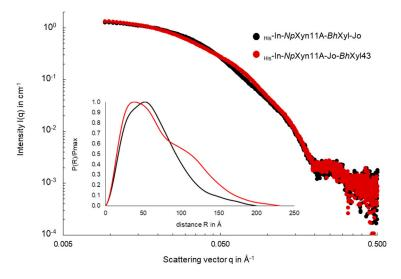
**Figure 2.** Superimposition of SAXS data from <sub>His</sub>-In-*Np*Xyn11A-*Bh*Xyl43-Jo and <sub>His</sub>-In-*Np*Xyn11A-Jo-*Bh*Xyl43 constructs (black and red dots respectively). The data are presented as a plot of Log I(q) in  $cm^{-1}$  vs. Log q in Å<sup>-1</sup> to magnify the region of small angles. In the box below is represented the pair distribution function p(r) of each form, plotted as a function of P(r)/Pmax vs. r in Å.
