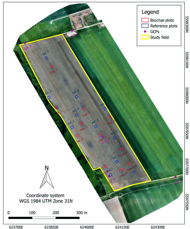
Fig. 1. The experimental area within the chicory field revealing the composition of the 11 pairs of biochar-enriched versus reference plots as well as the location of the ground control points. Century-old biochar-enriched patches are visible as darker black ovals. An RGB orthomosaic image captured by the unmanned aerial vehicle on the 22th May of 2018 is used as the background.
