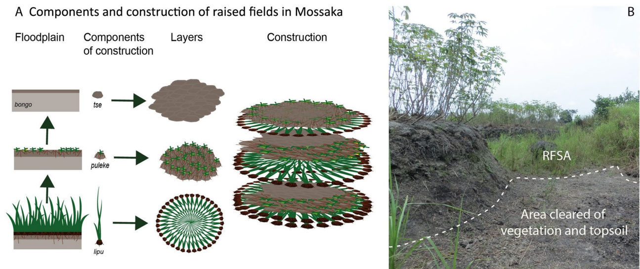
Figure 2. Mode of construction of RFs in Mossaka. (A) Materials used to construct RFs, and sequence of placement. Lipu : earth clumps with rooted vegetation; puleke : topsoil with vegetation debris; tse : topsoil from the RFSA; bongo : grey clay (C horizon) (Illustration made with Adobe Illustrator). (B) Area cleared of vegetation and topsoil ( tse ) next to field N2 (which was planted with manioc). Photo (1–20 August 2017), Leonor Rodrigues.
