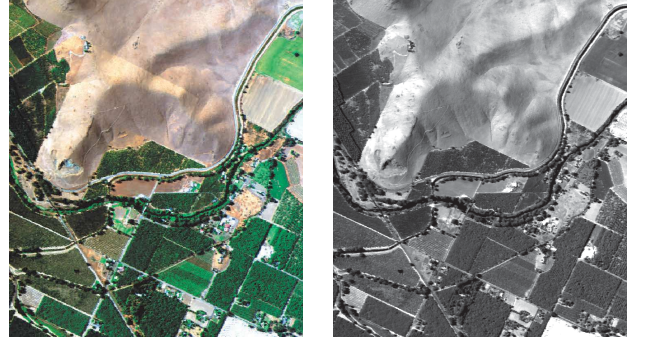
Fig. 6. AVIRIS image. Color composition of (Left) hyperspectral image and (Right) corresponding panchromatic image.
