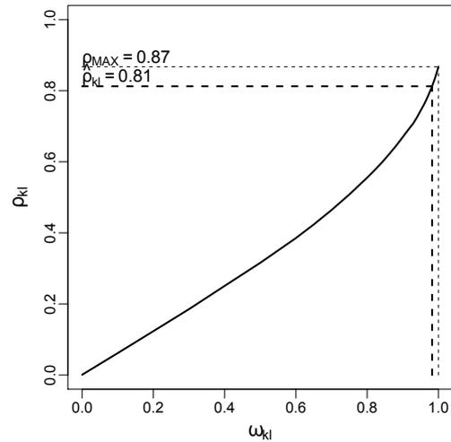
**Figure 2.** Illustration of the relationship between  $\omega_{kl}$  and  $\rho_{kl}$  for the month of July and for stations GOS and ANT. A Markov chain of order 4 is considered in this example. The correlation between the observed states is  $\hat{\rho}_{kl} = 0.81$  and can be reproduced using a bivariate Gaussian distribution with a correlation parameter of  $\omega_{kl} = 0.98$ . The maximum correlation  $\rho$  which can be obtained if  $\omega_{kl} = 1$  is  $\rho_{\text{MAX}} = 0.87$ .
