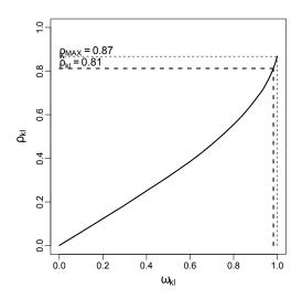
**Figure 2.** Illustration of the relationship between  $\omega_{kl}$  and  $\rho_{kl}$  for the month of July and for stations GOS and ANT. A Markov chain of order 4 is considered in this example. The correlation between the observed states is  $\hat{\rho}_{kl} = 0.81$  and can be reproduced using a bivariate Gaussian distribution with a correlation parameter of  $\omega_{kl} = 0.98$ . The maximum correlation  $\rho$  which can be obtained if  $\omega_{kl} = 1$  is  $\rho_{MAX} = 0.87$ .
