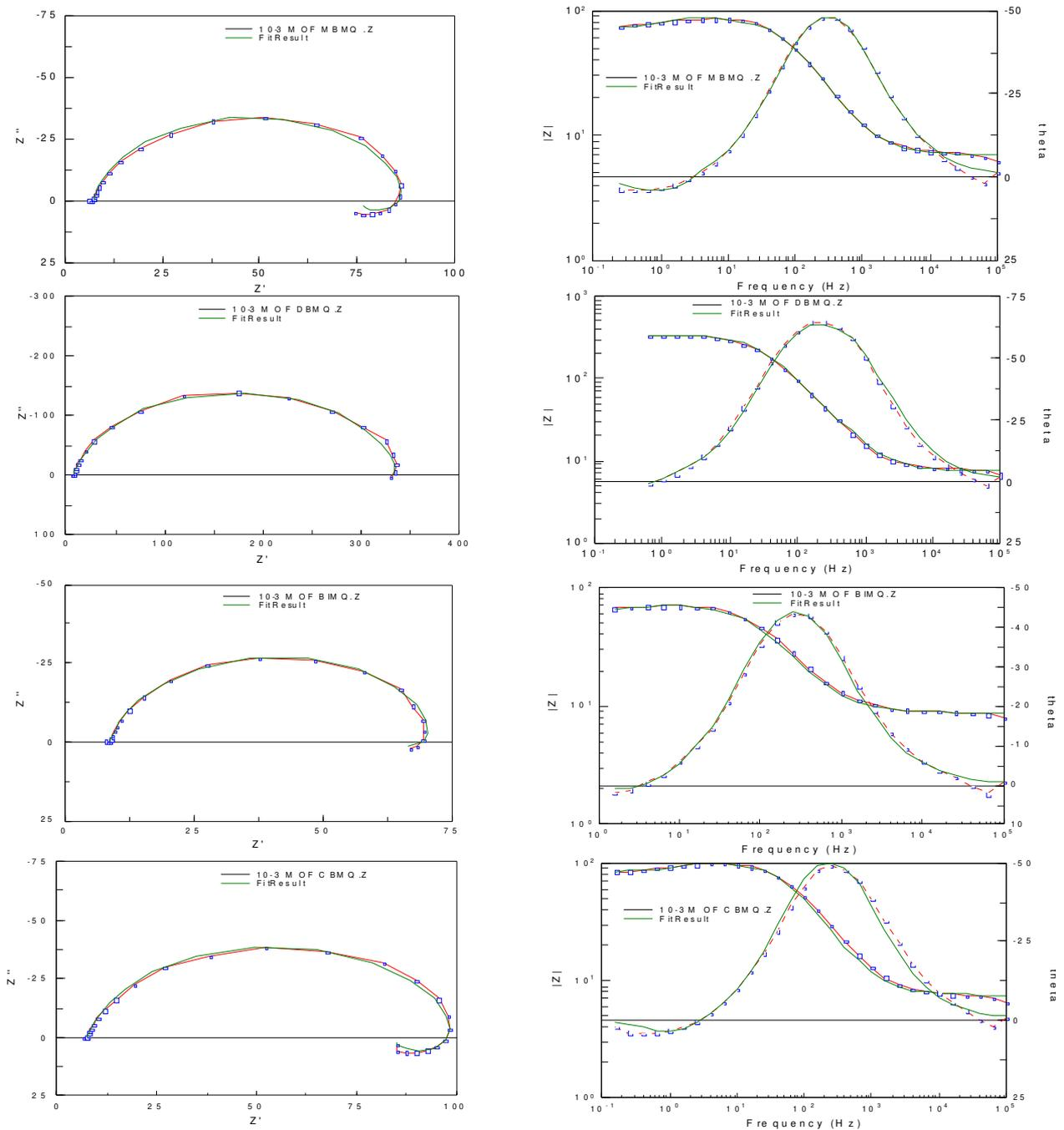
5 **Fig. 4.** EIS Nyquist and Bode diagrams for CS/2 M  $H_3PO_4$  +  $1 \times 10^{-3}$  M BIMQ, MBMQ,
