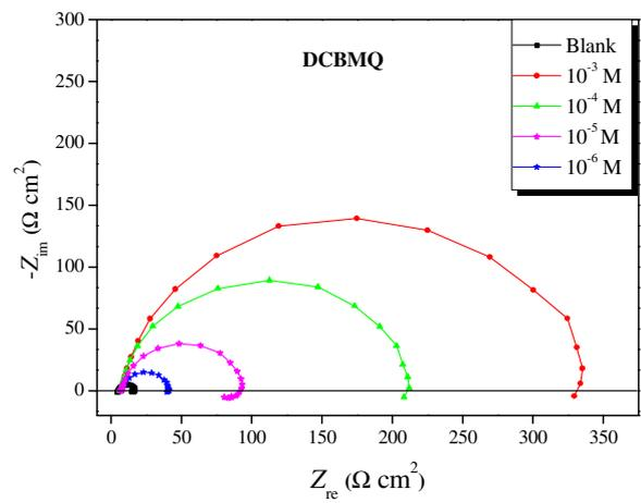
4 **Fig. 2.** Nyquist plots of the CS substrate in 2 M H<sub>3</sub>PO<sub>4</sub> with BIMQ, MBMQ, CBMQ and
