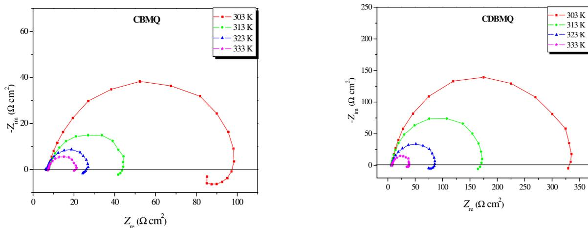
1 **Fig. 6.** Nyquist plots for CS in 2 M H<sub>3</sub>PO<sub>4</sub> medium containing 10<sup>-3</sup> M of various synthesized
