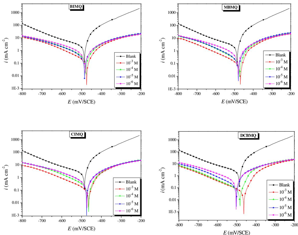
1 **Fig. 1.** Tafel plots for CS in 2 M H<sub>3</sub>PO<sub>4</sub> prior to and after adding of various concentrations of
