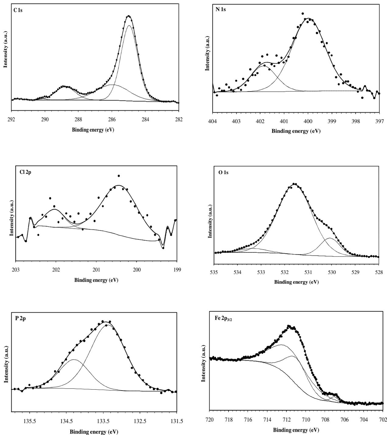
1 **Fig. 12.** High-resolution X-ray photoelectron deconvoluted profiles of C 1s, N 1s, Cl 2p,
