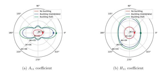
Figure 11: Polar diagram of the first component of matrices A and H for panel nº 7
