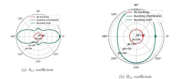
Figure 9: Polar diagram of the first component of matrices  $\mathbf{A}$  and  $\mathbf{H}$  for panel n<sup>o</sup> 1
