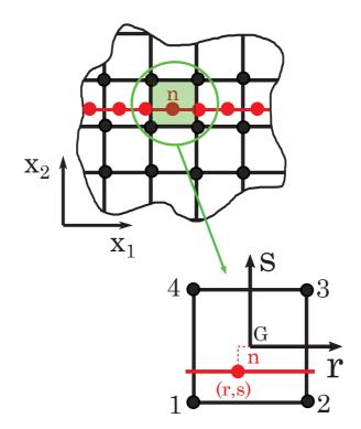
Figure 12: Differences between GFEM and LFEM meshes
