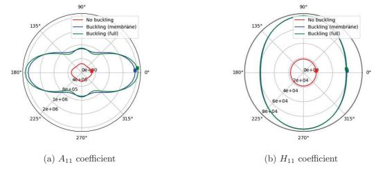
Figure 10: Polar diagram of the first component of matrices A and H for panel no 6
