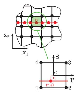
Figure 12: Differences between GFEM and LFEM meshes
