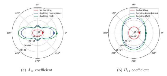
Figure 11: Polar diagram of the first component of matrices A and H for panel no 7
