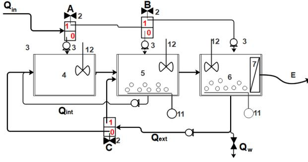
Fig. 1. Schematic diagram of the flexible platform.  $Q_{in}$ . influent; 2. Two position valve (position 1 or 0); 3. feed pump; 4. Anoxic tank; 5. Aerobic tank; 6. Aerobic tank; 7. Perfect membrane; E. Effluent;  $Q_{int}$ . Internal sludge recycling;  $Q_{ext}$ . external sludge recycling; 11. Air compressor; 12. Mechanical mixer;  $Q_w$ . Waste sludge.
