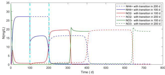
Fig. 2. Influence of retention time. Dynamic ammonium (blue), nitrate (green) and nitrite (red) concentrations for transitions at 100 days (continuous line) and at 200 days (dashed line)
