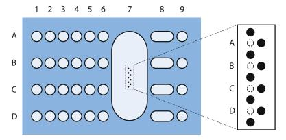
**Fig. 3** CellASIC<sup>®</sup> ONIX B04A microfluidic plate. Schematics of the plate. The plate is organized in four rows (A-D) allowing four independent experiments, and nine columns corresponding to: (1-5), wells for media/solutions; (6), wells for medium for cell loading; (7), area containing the four culture micro-chambers (A-D); (8), trashes, and (9), loading wells for the cells
