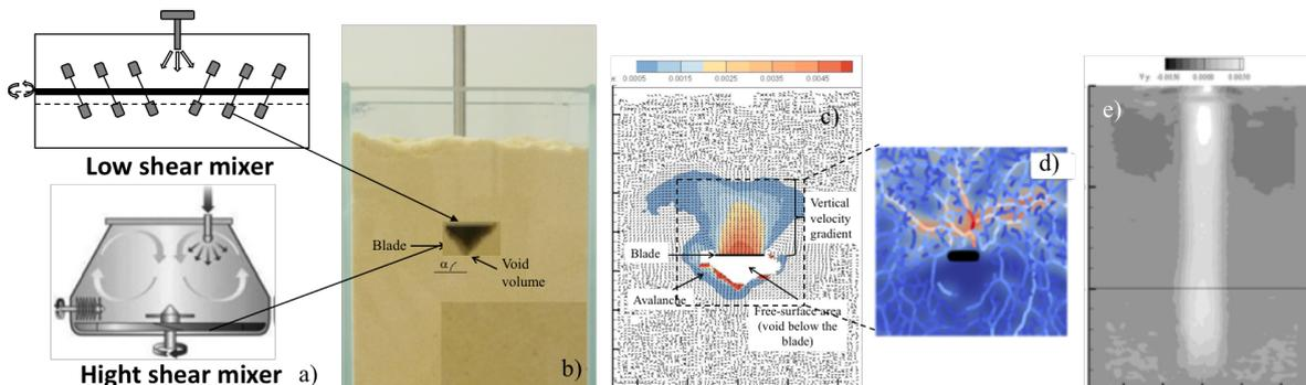
**Figure 1.** From reactors (a) to the experimental device (b) to identify particle mobilities by PIV (c) and DEM simulations (d) focused around the blade and the active and passive zones of mobilities in the granular medium (e).
