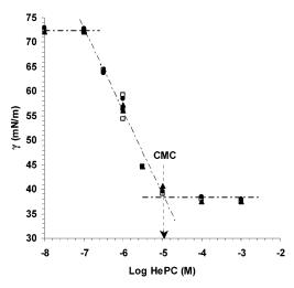
**Figure 4.** Interfacial behavior of HePC and HePC–AmB mixtures. Surface tension ( $\gamma$ ) was measured as a function of HePC concentration (molar), alone ( $\bullet$ ) or in a mixture with AmB at HePC/AmB molar ratios of 100 ( $\Box$ ) or 5 ( $\blacktriangle$ ). Measurements were performed in triplicate at 23 ± 2 °C.
