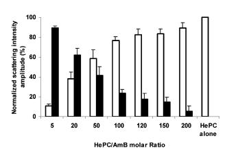
**Figure 5.** Normalized light scattering intensity amplitude as a function of HePC/AmB molar ratio. The AmB concentration was fixed at 10  $\mu$ M, and the HePC concentration was increased from 50  $\mu$ M to 2 mM. Two different populations were considered: mean diameter of 7 nm (white bars) and mean diameter of 210 nm (black bars). All measurements were expressed as means  $\pm$  SD of three determinations with three different samples (n = 9).
