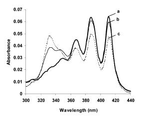
**Figure 2.** Effect of HePC at concentrations below its CMC on the absorption spectrum of AmB (total concentration of 1  $\mu$ M): (a) AmB alone in water, (b) HePC/AmB molar ratio of 4, and (c) HePC/AmB molar ratio of 8. The spectra were recorded 45 min after mixing and are representative of three experiments.
