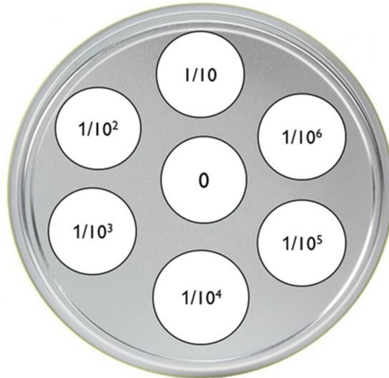
Fig 1. Schematic aspect of a serial dilution plate to determine the concentration of a bacterial suspension. 0 = 50 \mu l drop of undiluted bacterial suspension; 1/10-1/10 6 = 1/10-1/10 6 diluted drops of a bacterial suspension.
