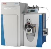
Injection of samples into nano HPLC coupled with Q-Exactive (Thermo Fisher Scientific)
