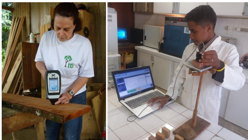
Fig. 18: Collecting NIR spectra with different portable spectrometers.
