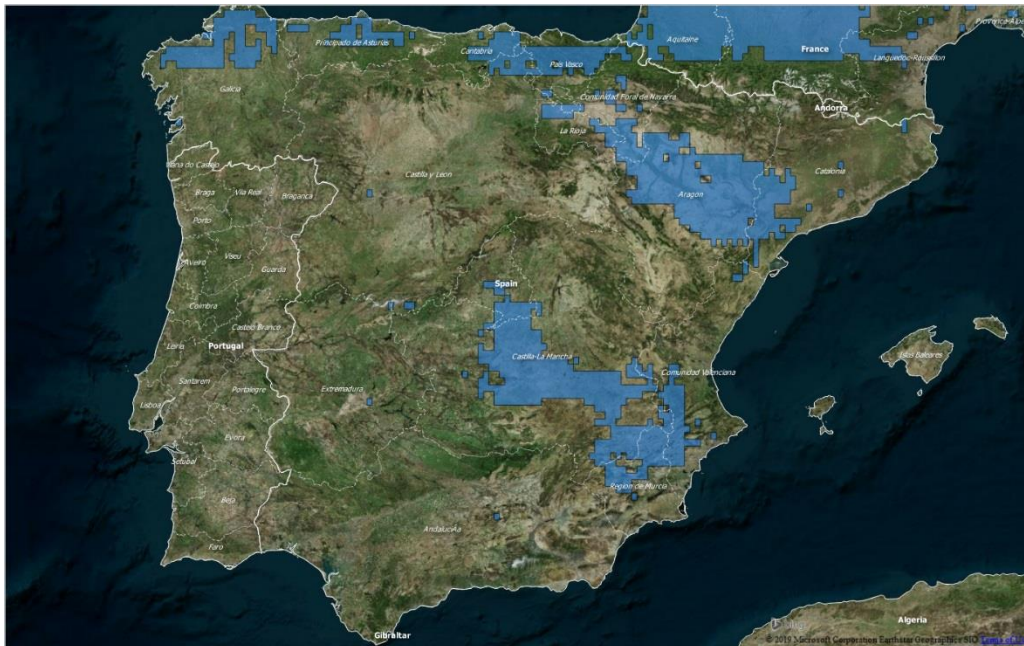
Fig. 15: Illustrative example of an isoscape result. Regions in Spain where the signature of a sample (declared as spruce from Spain) satisfied the 95% confidence interval of the isoscapes for D/H, ^{18}\text{O}/^{16}\text{O} , ^{13}\text{C}/^{12}\text{C} and ^{34}\text{S}/^{32}\text{S} .
