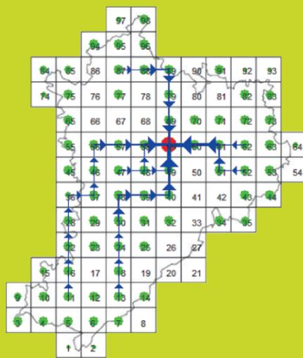
Biomass supply chain to an organosolv biorefinery in the Beauce region as derived from the optimisation modelling approach. Source: BIOCORE ■
