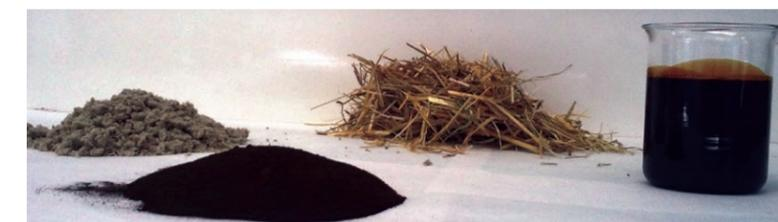
Figure 6 – From left to right: cellulose, lignin powder, wheat straw, C5 syrup. The CIMV technology allows extracting the cellulose, hemicellulose and lignin out of biomass. © CIMV ■
