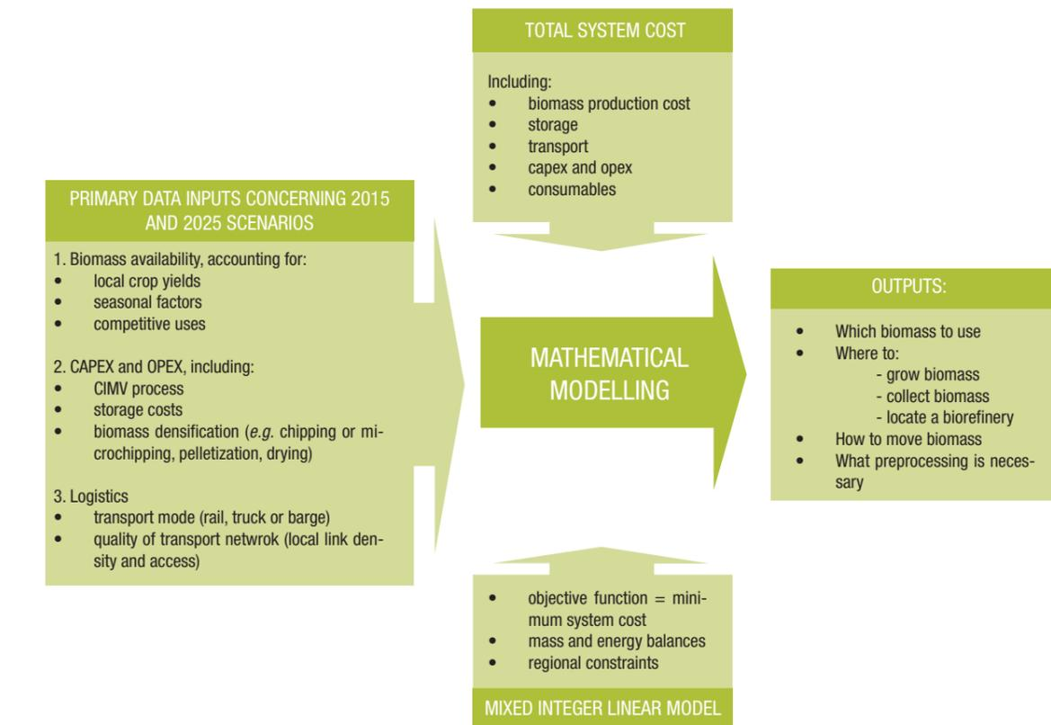
Figure 11 – Objective-driven modelling framework used to design the biomass supply chain in BIOCORE's case studies. © IMPERIAL
