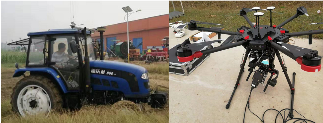
Fig. 1. Precision agriculture (PA) equipment developed for farm management. For example, high precision positioning systems, laser land levelling, precision seeding/fertilizer/irrigation/harvesting and satellite images. Shown here is the GNSS tractor and UAV developed by the PAFiC project ( http://ceg-pafic.ncl.ac.uk/index.php/en/ ).
