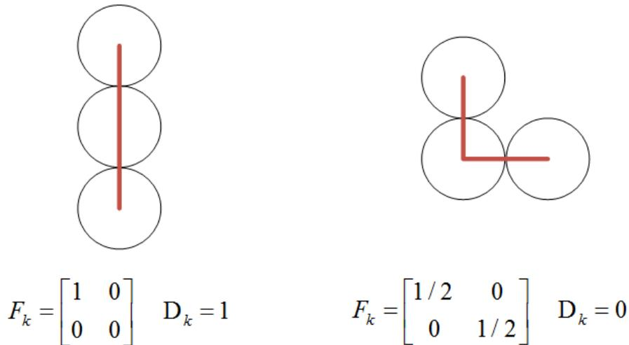
Figure 12: Extremal conditions of force chain linearity  $D_k$ .
