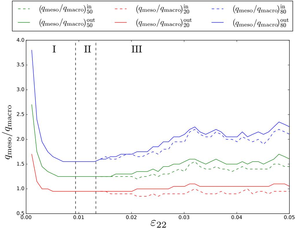
Figure 10: Evolution of the 20 % (lower), 50 % (middle) and 80 % (upper) passing fractions of the cumulative distribution of  $q_{\text{meso}}/q_{\text{macro}}$  during biaxial loading for the dense specimen. After the stress peak, cumulative distributions are computed separately inside (dashed) and outside (solid) of the shear band.  $q_{\text{meso}}$  is computed based on  $\sigma_{\Omega_{3-p}}^{\text{max}}$  (see Section 2.3)
