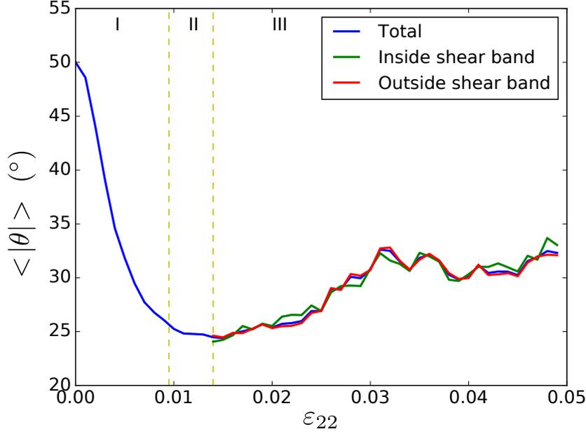
Figure 23: Evolution of the mean non coaxial angle  $\langle |\theta| \rangle$  during the biaxial test for the dense sample. As the shear loading develops,  $\langle |\theta| \rangle$  is computed separately inside and outside the shear band.
