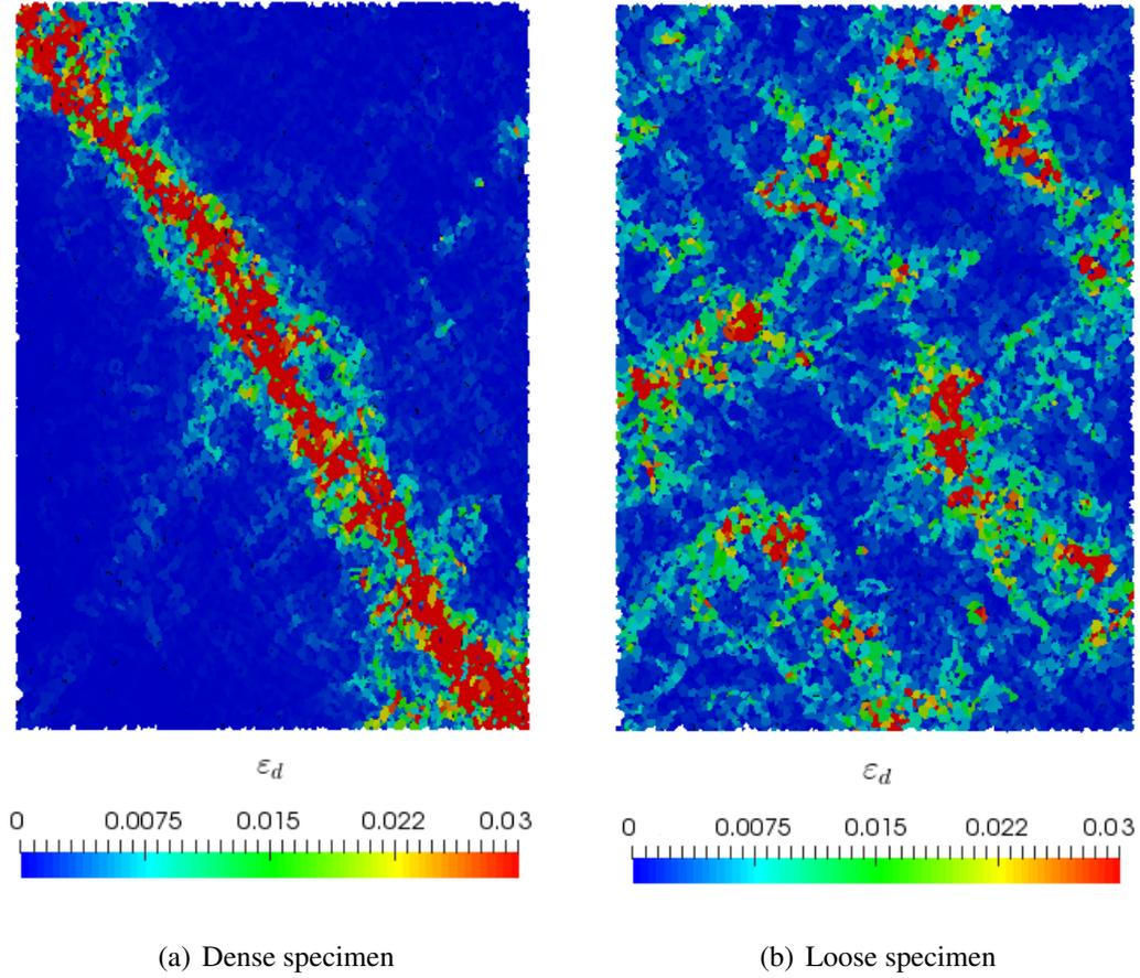
Figure 5: Spatial distributions of incremental deviatoric strains  $\varepsilon_d$  for dense (a) and loose (b) specimens during biaxial tests at  $\varepsilon_{22} = 0.03$ . Local incremental strains are computed with macroscopic strain increments  $d\varepsilon_{22} = 10^{-3}$ .
