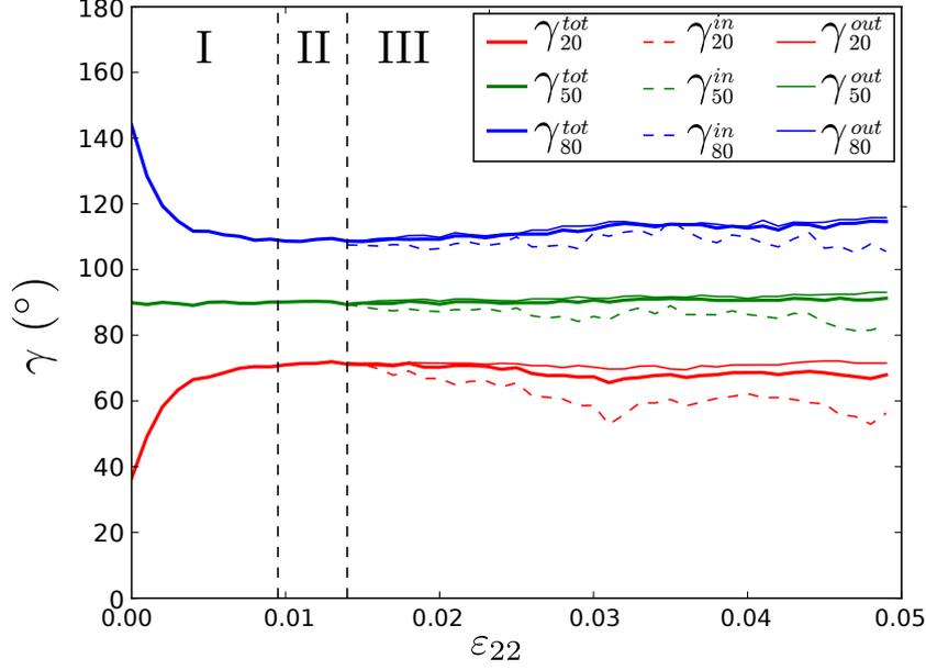
Figure 21: Strain evolution of the 20 %, 50 % and 80 % passing fractions of the cumulated distributions of the geometrical orientation  $\gamma$  of 3-p groups. After the stress peak, cumulative distributions are computed separately inside and outside the shear band.
