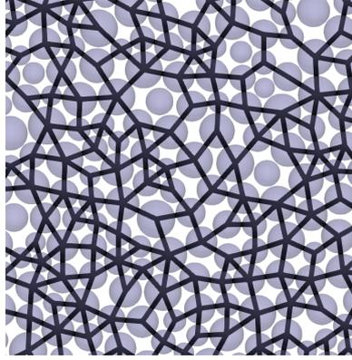
Figure 3: An example of 2D loop tessellation in granular materials
