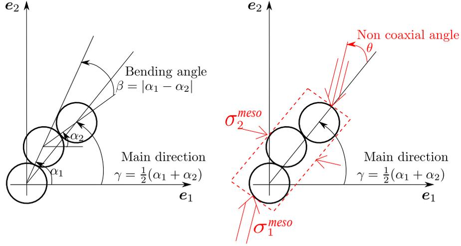
Figure 17: Geometrical and mechanical features of 3-p groups. The geometry is characterized by the bending angle  $\beta$  and orientation angle  $\gamma$  while the mesoscopic stress state is characterized by the major ( $\sigma_1$ ) and minor ( $\sigma_2$ ) stresses as well as the non coaxial angle  $\theta$ .
