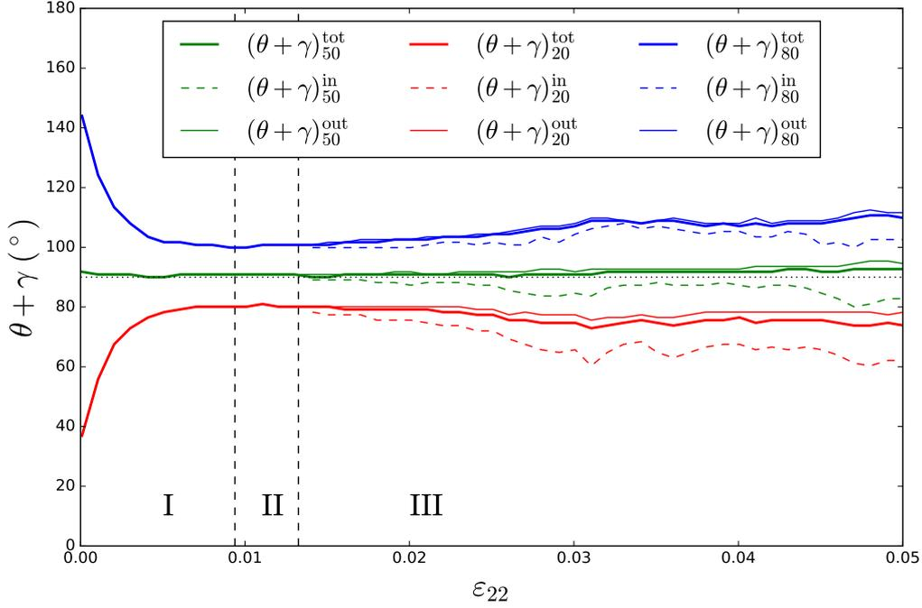
Figure 22: Strain evolution of the 20 %, 50 % and 80 % passing fractions of the cumulated distributions of the principal stress direction orientation  $\gamma + \theta$  of 3-p groups. After the stress peak, cumulative distributions are computed separately inside and outside the shear band.
