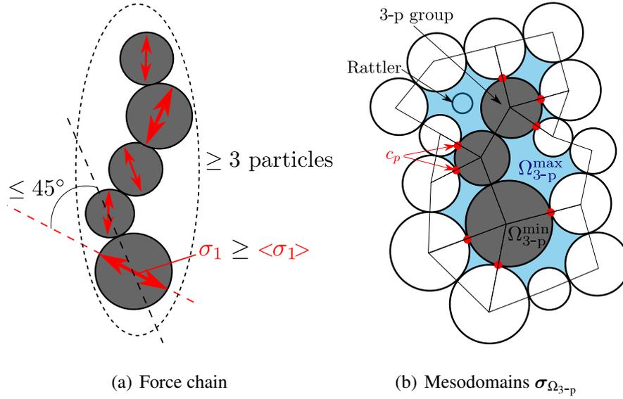
Figure 6: Definition of (a) a force chain according to Peters et al. (2005) and (b) the two mesodomains  $\sigma_{\Omega_{3-p}^{\min}}$  (3-p group in grey) and  $\sigma_{\Omega_{3-p}^{\max}}$  (3-p group in grey and pore space in light blue). Contact points  $c_p$  involved in Equation (4) are shown as red dots.
