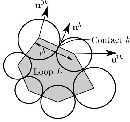
Figure 4: Mesostrain definition of a loop domain  $L$ .
