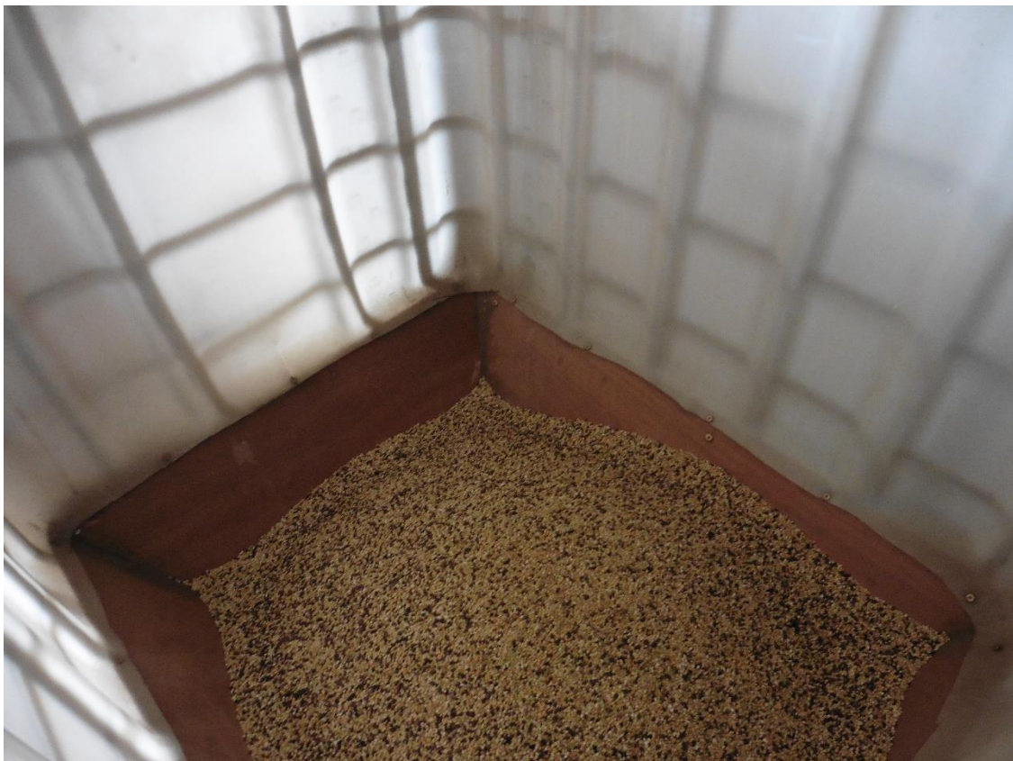
Mix of dehulled (bright) and un-dehulled seeds (dark) before optical screening
