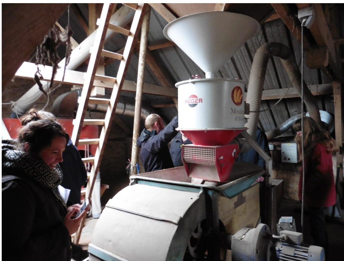
The Heger (Moulins d'Alma) dehulling centrifuge and the winnowing machine below (Tarare) used for the first wind screening
