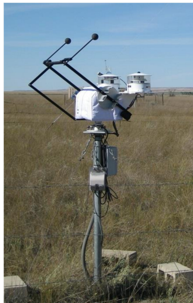
Figure 3. Example of pyranometer for measuring diffuse radiation. An accurate sun-tracker is installed to shield the pyranometer from direct solar beam. Photo is courtesy of surface radiation budget network (SURFRAD) US-FPK site.
