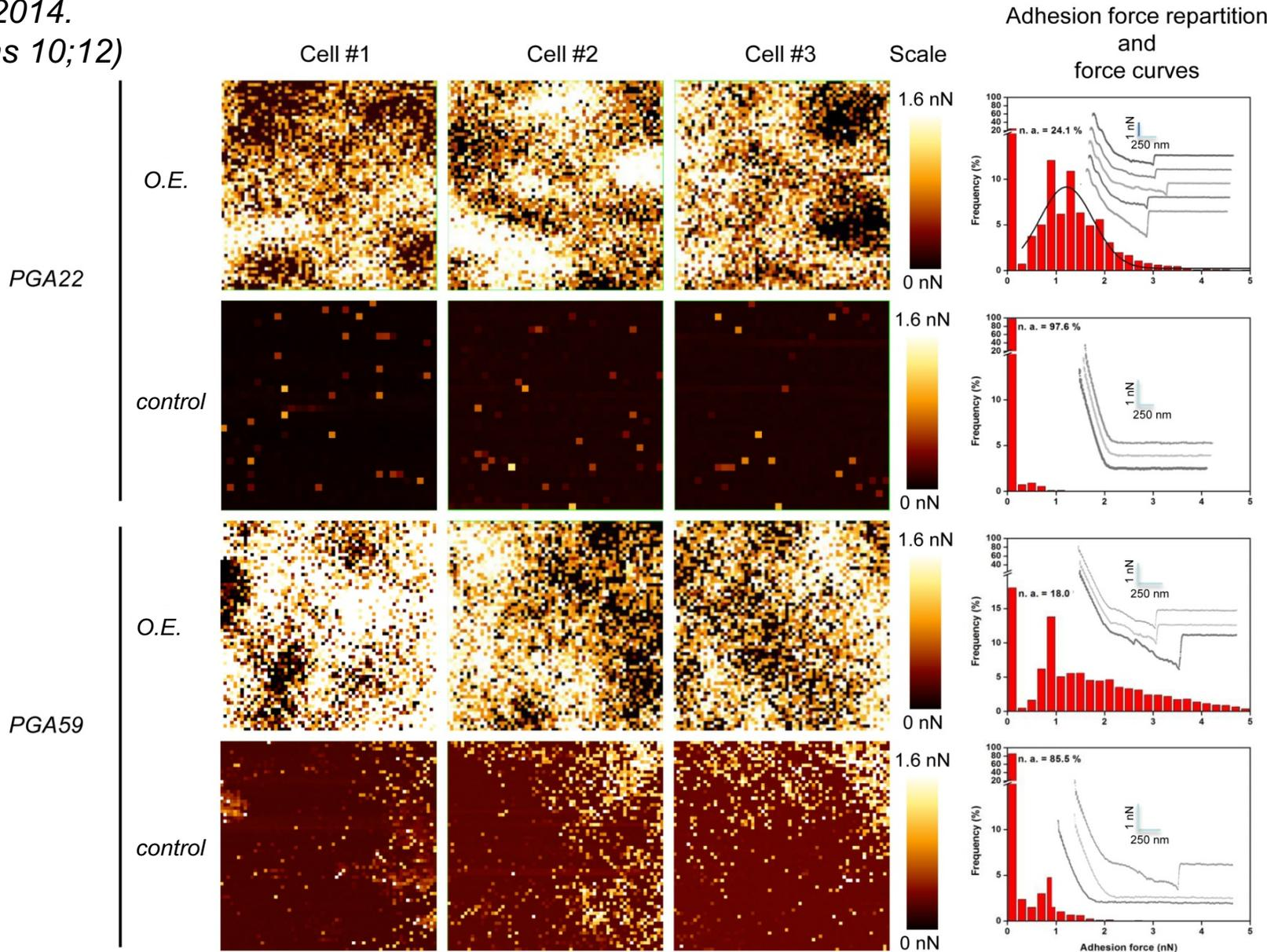
***AFM allowed us to unravel the morphologic effect on yeast cells of Heat Shock, Osmotic Shock, exposure to toxins and drugs.***
