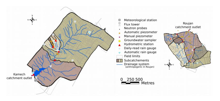
Hydrometeorological monitoring infrastructure. The different surface colors indicate the subcatchments delineated from hydrometric stations. In the Roujan catchment, the drainage system contains mainly anthropogenic ditches, fed by surface runoff. In the Kamech catchment, the drainage system consists mainly of a network of natural wadis and permanent gullies.
