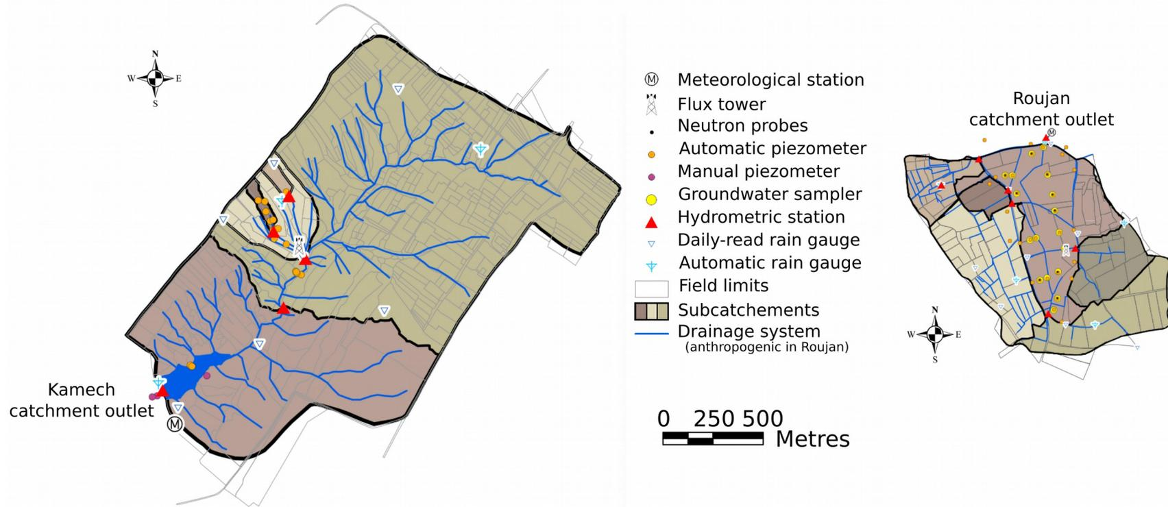
*Hydrometeorological monitoring infrastructure. The different surface colors indicate the subcatchments delineated from hydrometric stations. In the Roujan catchment, the drainage system contains mainly anthropogenic ditches, fed by surface runoff. In the Kamech catchment, the drainage system consists mainly of a network of natural wadis and permanent gullies.*
