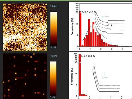
Adhesion force Maps of  $1\mu\text{m}^2$ , corresponding histograms representing the adhesion force repartition, and a few representative force curves.
