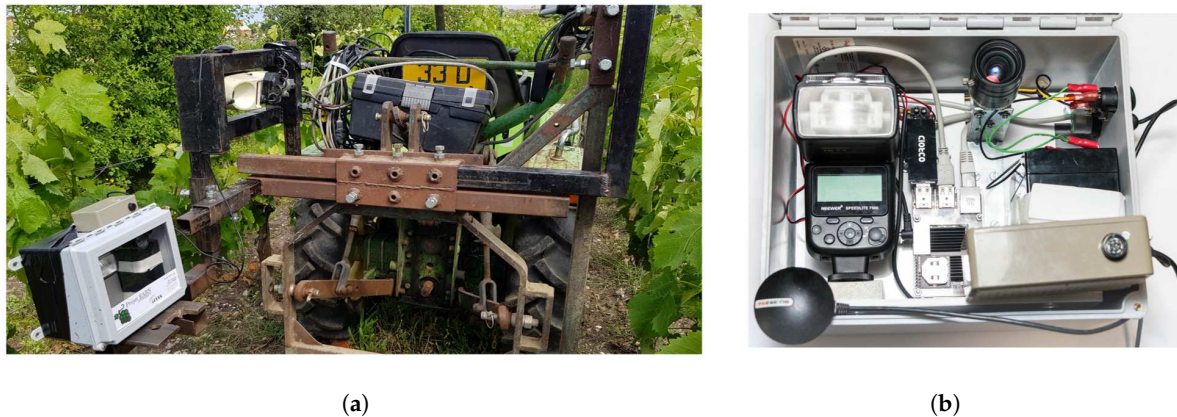
Figure 1. Instrumentation: an autonomous in-field imaging sensor, (a) a device embedded on a vine tractor and (b) details and elements of the device.
