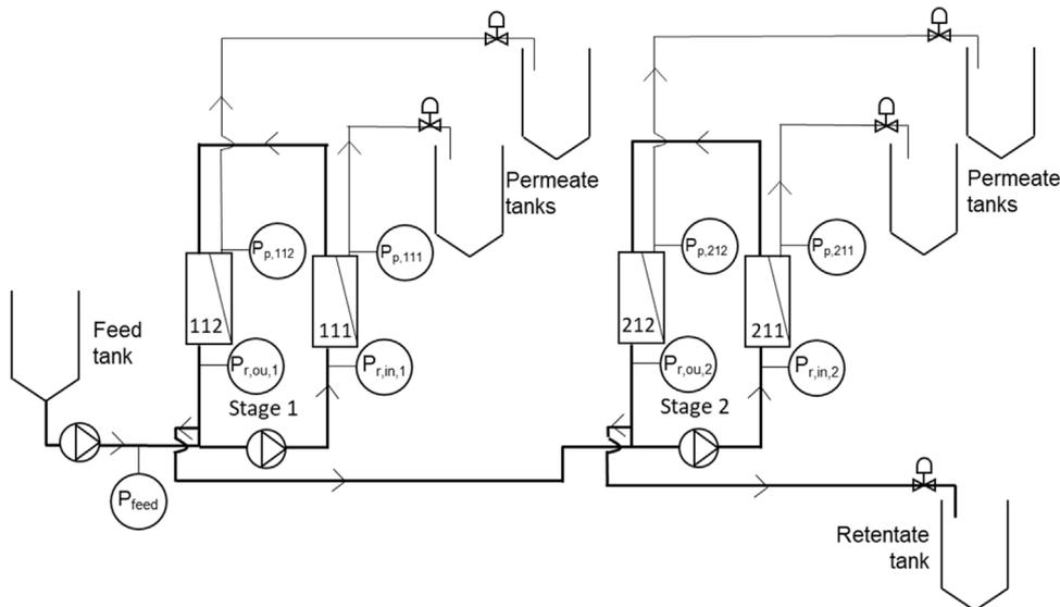
**Fig. 5 – Locations of pressure sensors in (a) an industrial plant and (b) experimental pilot. Example of gradient of permeability membrane technology with two stages and one line in parallel, with two modules in series in each stage.**
