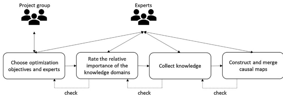
**Fig. 1 – The formulation method applied to the microfiltration multiobjective optimization problem (adapted from Hobballah et al. (2018)).**
