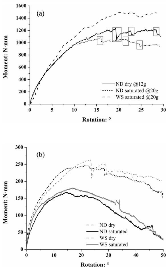
**Fig. 8** Push-over curves of two types of model roots from (a) centrifuge and (b) 1-g testing in different water conditions (prominent drops in ND centrifuge tests are marked by boxes, results at model scale)
