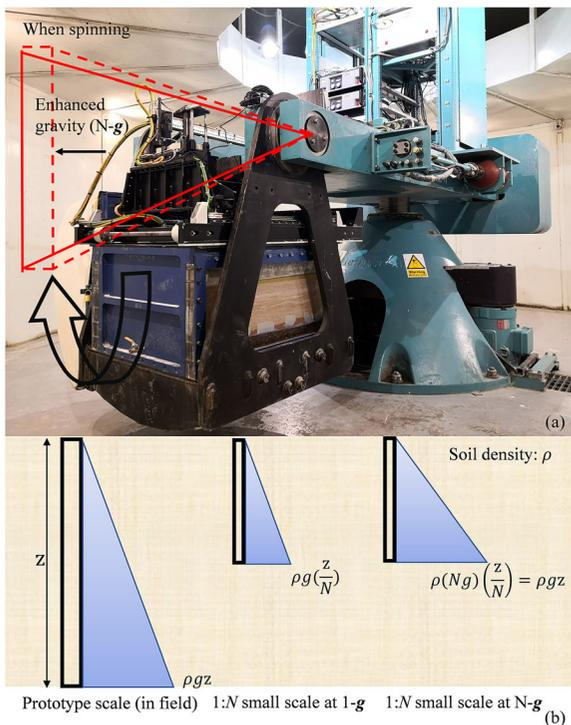
**Fig. 3 Centrifuge technology:** (a) beam centrifuge at the University of Dundee, UK; (b) vertical stress of structure buried in the soil under different scales and *g*-levels (red drawing is the position of the centrifuge basket when spinning)
