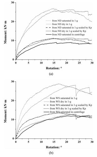
Fig. 11 Comparison of rotation-moment curve at prototype derived from 1-g and centrifuge testing: a model ND; b model WS
