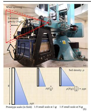
Fig. 3 Centrifuge technology: (a) beam centrifuge at the University of Dundee, UK; (b) vertical stress of structure buried in the soil under different scales and *g*-levels (red drawing is the position of the centrifuge basket when spinning)
