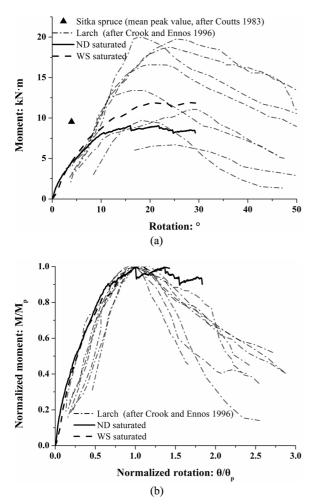
Fig. 10 Moment-rotation curve of two model roots transferred into prototype, with comparison with some in field testing results: a in absolute value; b in normalized value
