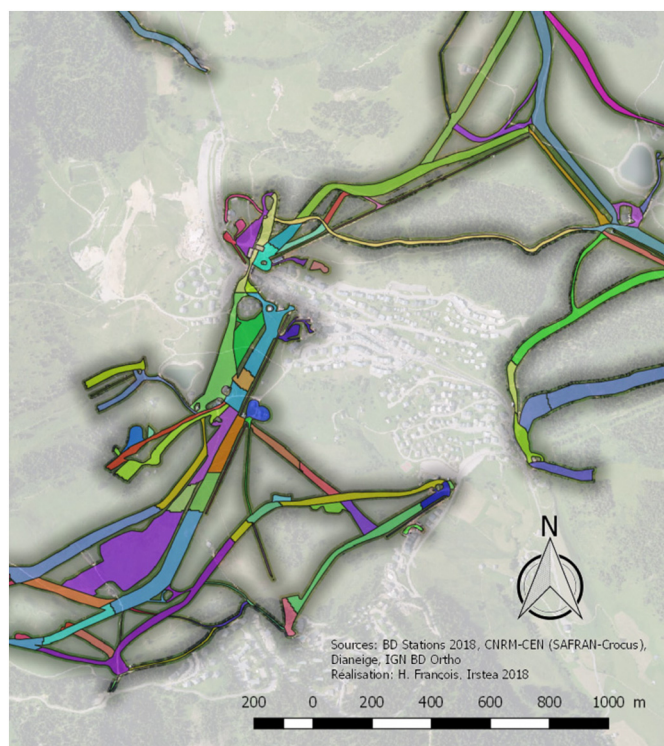
Fig. 3. Example of the discretization of a ski resort (Les Saisies) into SRUs based on the topographic characteristics of the slopes and the presence/absence of snow guns. SRU colors were chosen arbitrarily for visualization purposes.
