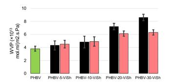
Fig. 8 Water vapor permeability (WVP) in PHBV-based biocomposites with ViSh-V (■) and ViSh-G (■) fillers
