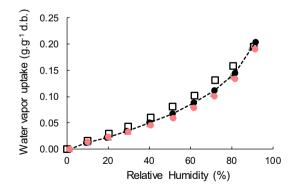
**Fig. 3** Water vapor sorption isotherm of ViSh-V ( $\bullet$ ), ViSh-C ( $\triangle$ ), ViSh-G ( $\bullet$ ) and cellulose ( $\square$ ) (data for cellulose are from [41], standard deviation bars are not visible as they are lower than the symbol size)
