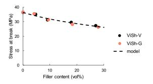
Fig.7 Pukánszky's model applied for ViSh-V and ViSh-G based composites
