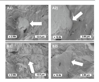
Fig. 4 SEM pictures of cryo-fractured sections: (A1-2) PHBV-20ViSh-V, (B1–B2) PHBV-20ViSh-G. White arrows show the matrix/filler interface
