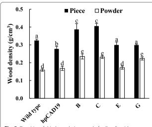
**Fig. 5** Densities of dried wood pieces and of cell wall residues (powders) prepared from the stem of each line. Three biological replicates were used in the analysis. Different letters indicate statistically significant differences between the various lines at P < 0.01 determined by one-way ANOVA followed by Tukey multiple comparison tests. Error bars indicate the standard deviation
