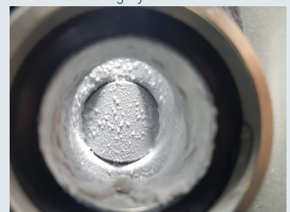
Sensor-measured in-pipe milk fouling.
