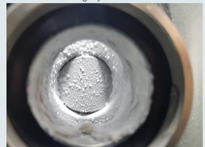
Sensor-measured in-pipe milk fouling.
