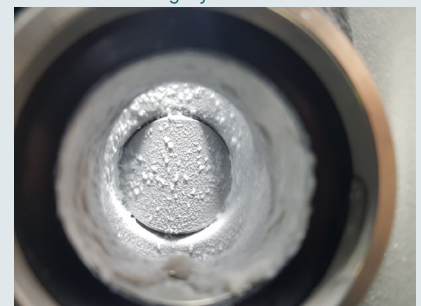
Sensor-measured in-pipe milk fouling.
