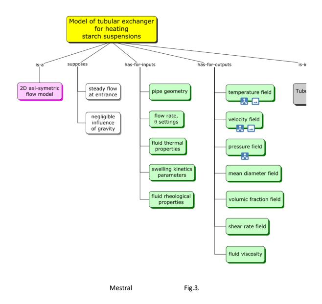
**Figure 3**: Concept map adapted to the representation of the model, taking the model of "Heat exchanger for starch suspension", for example. Note that a concept "simulator" is added on the right to represent how the model is implemented and to give access to the results computed by the model. A knowledge sheet may be opened from this Cmap using the icons, providing information about the theoretical framework on which the model is based.
