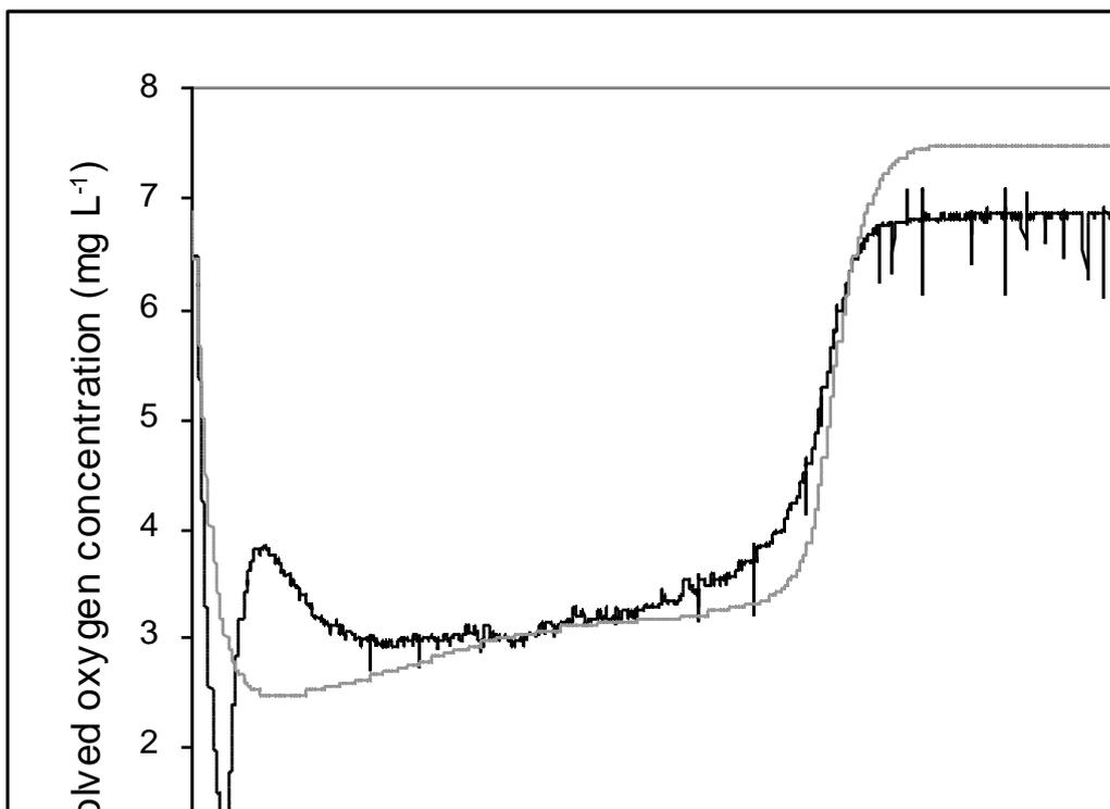
**Figure 5.** Dissolved oxygen concentration for a respirometric assay (initial ammonia concentration 50 mg N-NH<sub>4</sub><sup>+</sup>/L, initial nitrite concentration 15 mg N-NO<sub>2</sub><sup>-</sup>/L; e: experimental value, m: model prediction).
