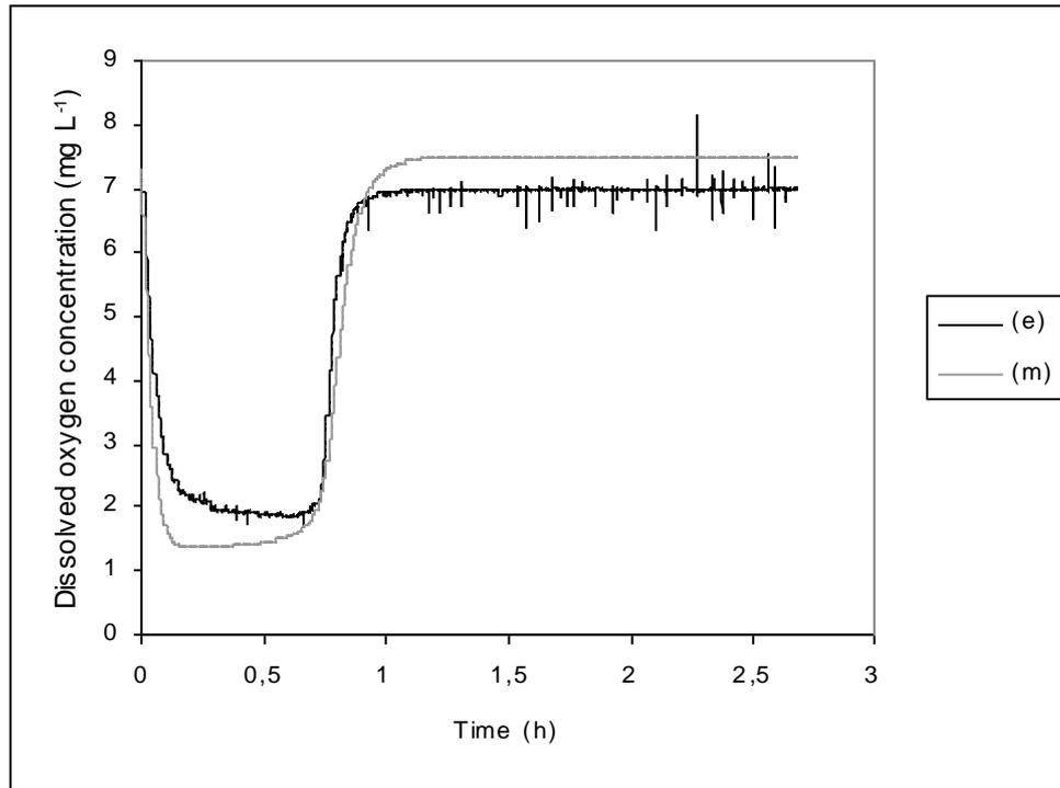
**Figure 3.** Dissolved oxygen concentration in a respirometric assay at initial nitrite concentration of 60 mg N-NO<sub>2</sub><sup>-</sup>/L (e: experimental value; m: model prediction).
