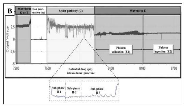
**Figure 1.** Electropenetrography device (A). The recorded waves (B) were: F - mechanical stress (derailment of the stylets); G - trophic stress (sap ingestion); NP - non-penetration of the stylets; C - search (extracellular paths); E - phloem activity (E1 - salivation; E2 - ingestion). pd - "potential drop": it can be subdivided into three subphases (II-1, II-2 and II-3).
