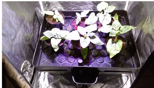
Fig. 10. Growing chamber of sunflower plants equipped with horticultural lamp, ventilation system and tide tank.
