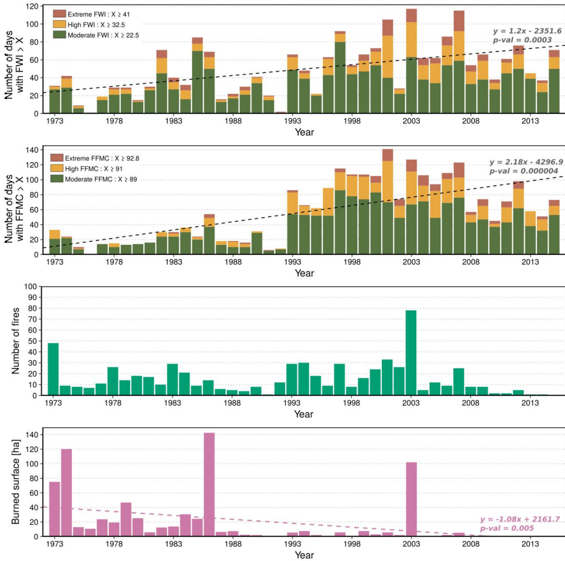
Figure 8 : Annual number of days with Fire Weather Index (FWI) and Fine Fuel Moisture Code (FFMC) exceeding thresholds, number of fires and burned surface on Brague catchment DEMO over the period 1973-2015. The temporal linear trend is shown with a dashed line if significant (the sum of all days of moderate to extreme fire weather is taken into account for FFMC and FWI temporal trends).
