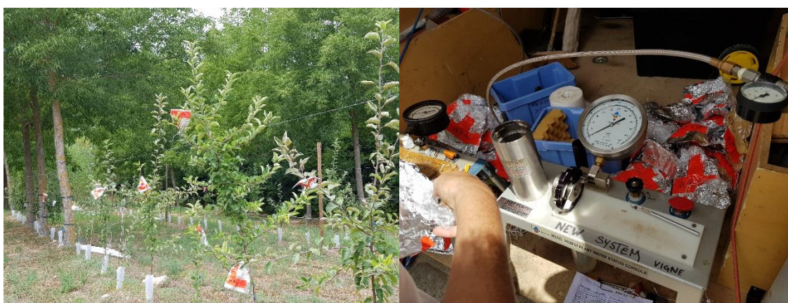
Photograph 3: Apple trees with the leaves for midday water potential inserted in the plastic bag covered in aluminium foil (left) and one of the two pressure chambers used for the measurement of water potential in the leaves (right).
