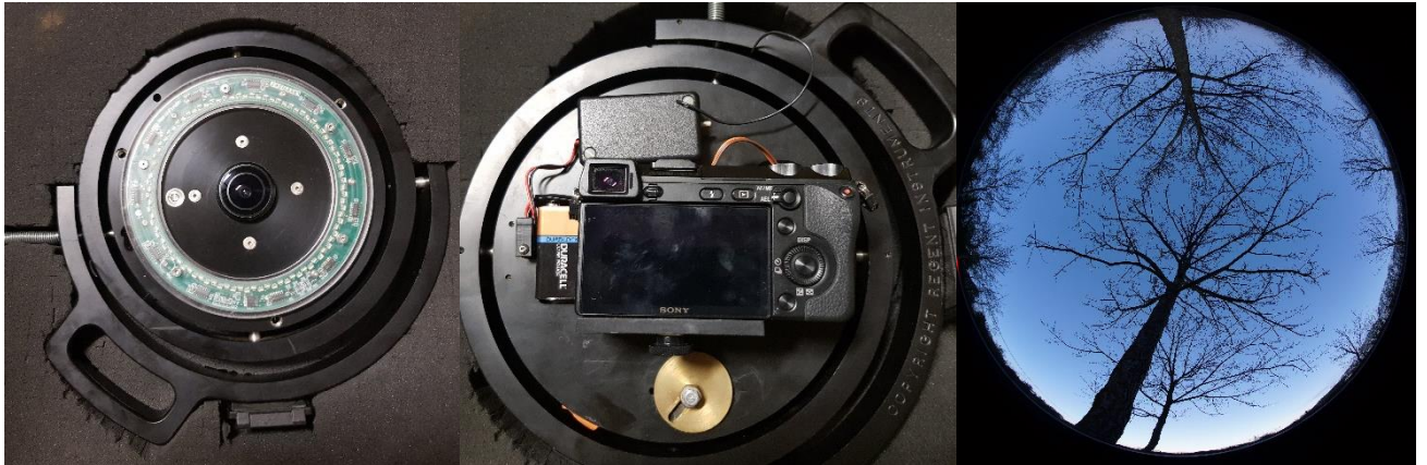
Photograph 2: 180° fisheye lens (left) and Sony camera (middle) used to take hemispheric photographs (right). The camera and lens were provided and calibrated by Regent Instruments Inc.
