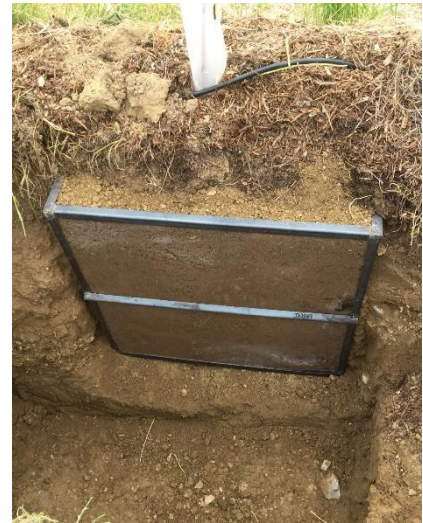
Photograph 4: In situ rhizotron in the apple-agroforestry experiment on plot A1 of the “domaine de Restinclière” (picture by Benjamin Pitchers).
