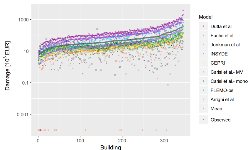
Figure 8. Observed damage vs. individual estimates of the monetary damage for the subset of buildings with claims. Data are ordered according to increasing value of mean estimate (in black).
