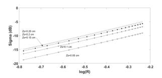
Fig. 3. Relationship between backscattering *IEM* simulations and log(R) for different  $Z_s$  (roughness parameter) levels
