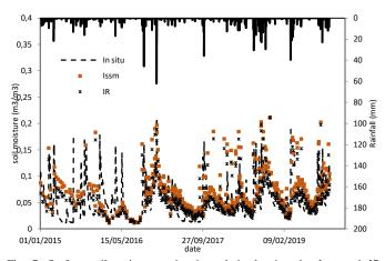
Fig. 7. Surface soil moisture estimations derived using the  $I_{SSM}$  and IR products compared with  $in\ situ$  measurements of soil moisture at the Barrouta site
