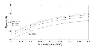
Fig. 2. Relationship between backscattering *IEM* simulations and soil moisture for different  $Z_s$  (roughness parameter) levels
