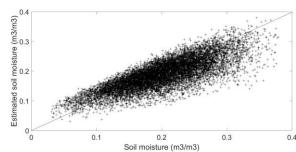
Fig. 6. Comparison between the input (actual) soil moisture used for the *IEM* simulations with variable roughness and the soil moisture estimations computed using two different indices: a)  $I_{SSM}$  and b) IR.
