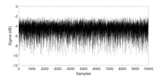
Fig. 4. IEM-simulated series for soil moisture ranging between 0 m<sup>3</sup>/m<sup>3</sup> and 0.4 m<sup>3</sup>/m<sup>3</sup>, a rms height equal to 0.8 cm, and a correlation length equal to 6 cm.
