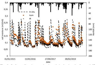
Fig. 8. Surface soil moisture estimations derived using the  $I_{SSM}$  and IR products compared with  $in\ situ$  measurements of soil moisture at the INGC site.
