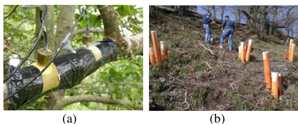
Fig. 2. Soil and plant monitoring at Monte Faito, Naples. (a) High-capacity tensiometers installed on chestnut. (b) Installation of TDR probes and conventional tensiometers in the ground (12/04/2018).
