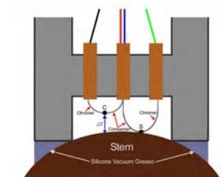
**Fig. 4.** PSY1 Stem Psychrometer schematic layout [18].
