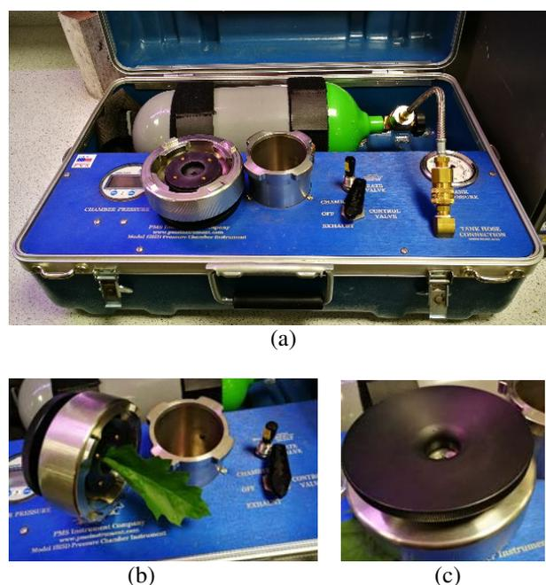
**Fig. 6.** (a) PMS 1515D Scholander Pressure Chamber. (b) Leaf inserted into the sealing ring. (c) Sealing ring mounted on the pressure chamber.
