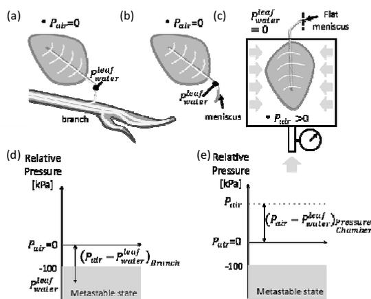
**Fig. 3.** Working principle of the Pressure Chamber (PC) technique for measurement of leaf water pressure. (a) leaf on the tree (water pressure is negative); (b) leaf excised (curved meniscus forming at the end of petiole); (c) air pressure increased around leaf (meniscus becomes flat).
