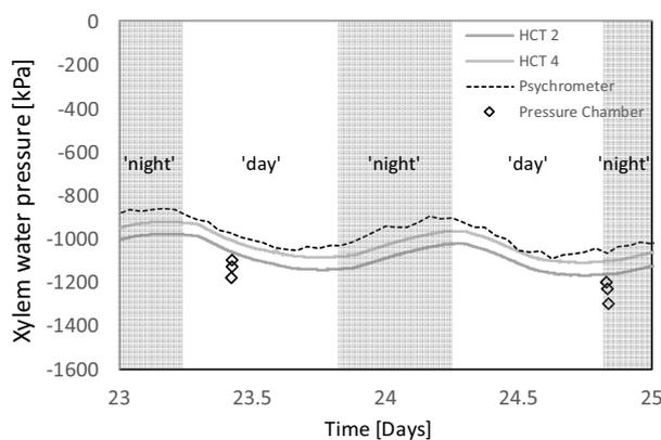
**Fig. 10.** Measurement of xylem water pressure using HCT2, HCT4, and transistor psychrometer (at 115 mm, 250 mm 400 mm above soil surface respectively) and pressure chamber (on leaves excised from tree branches).
