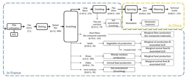
Figure 2. Process flow diagram illustrating the fate of the co-products from the production of a flax fiber technical textile. Boxes represent induced processes while dotted lines represent avoided processes
