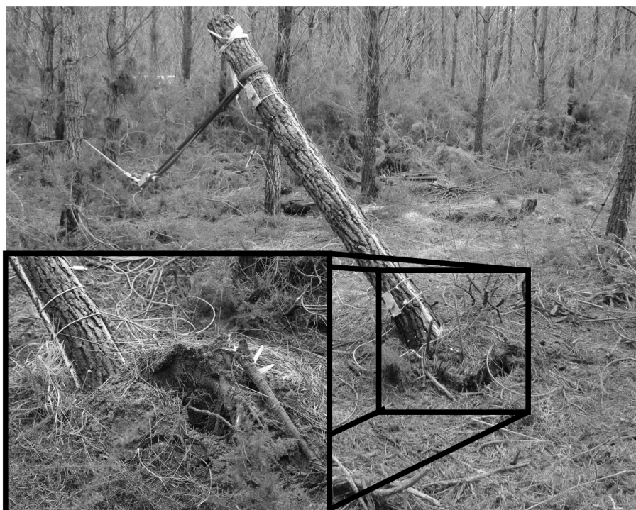
Figure 2: Root system after winching test. The zoom focus on the roots in the counterwinch sector that were pulled out the soil.
